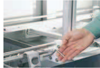
All the tanks can be emptied by pressing a lever. The bottom seals and level pipes are closed automatically when the machine is about to fill.
