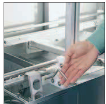
All the tanks can be emptied using a single lever. Bottom seals and level pipes are closed automatically when the machine is about to fill.
