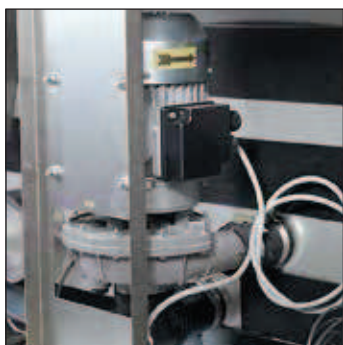
Improved hygiene with selfemptying pumps in wash and rinse zones.
